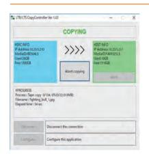
Installed on a computer connected via Ethernet to two LTS units, enables LTO tape files to be copied from either unit.
